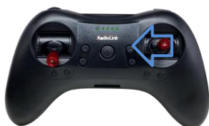
Roll stick to left, F121 flies to the left side
