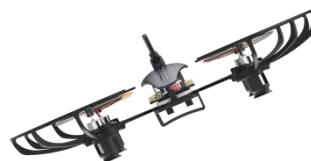
Roll stick to left, F121 flies to the left side
