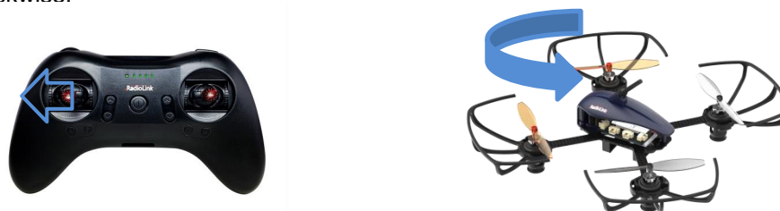
Yaw stick to the left , F121 turns anticlockwise
