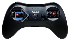
Yaw stick to the right, F121 turns clockwise
