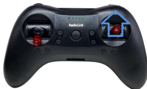
Pitch stick upward, F121 moves forward
